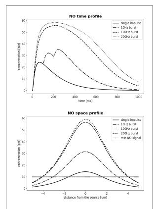
Fig. 3. Upper panel: Time profile of NO signal generated by a single source stimulated at different frequencies. The burst length is fixed at 200 ms. The observational point is located at 200 nm at the source. Bottom panel: Space profile of NO signal generated by a single source stimulated at different frequencies. All curves are referred to t = 210 ms. We reported the minimum concentration at 10 pM that is able to trigger NO dependent effects [7]
